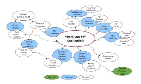
Figure 1: Resource Tree for Thermal Equipment
