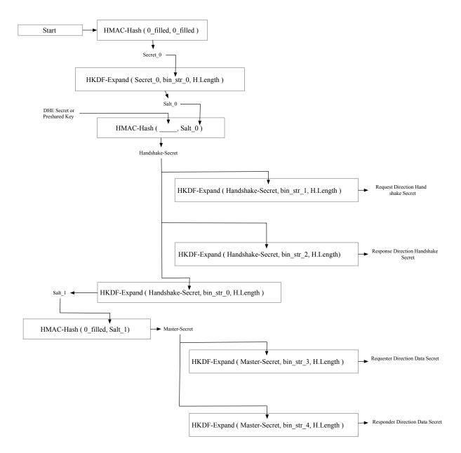
In the figure, arrows going out of the box are outputs of that box. Arrows going into the box are inputs into the box and point to the specific input parameter they are used in. All boxes represent a single function producing a single output and are given a name for clarity.
