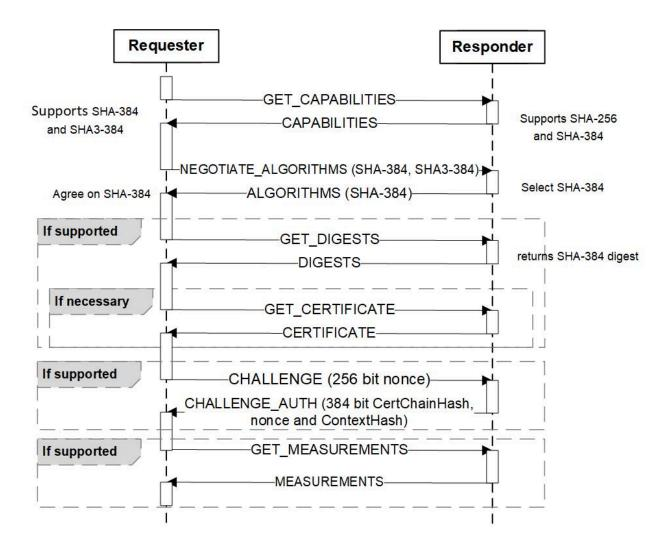
The SPDM protocol accounts for the possibility that both endpoints may issue **NEGOTIATE\_ALGORITHMS** request messages independently of each other. In this case, the endpoint A Requester and endpoint B Responder communication pair may select a different algorithm compared to the endpoint B Requester and endpoint A Responder communication pair.
