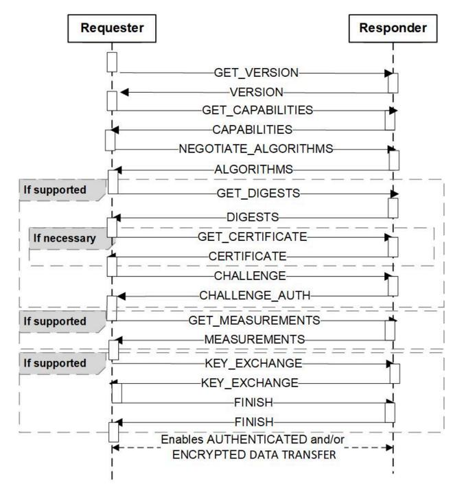
All SPDM request-response messages share a common data format, that consists of a four-byte message header and zero or more bytes message payload that is message-dependent. The following clauses describe the common message format and SPDM messages details each of the request and response messages.
