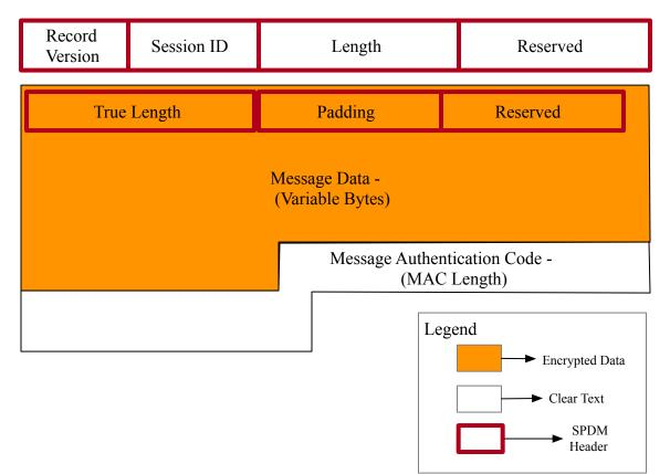
A record shall contain the complete cipher text as produced by a single invocation of AEAD\_Encrypt using the appropriate encryption key for the given direction of transmission, the appropriate per-record nonce and the selected AEAD Cipher Suite in ALGORITHMS.
