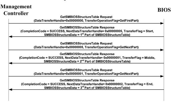
Figure 2 – Multipart SMBIOS Structure Table Transfer Using the GetSMBIOSStructureTable Command
