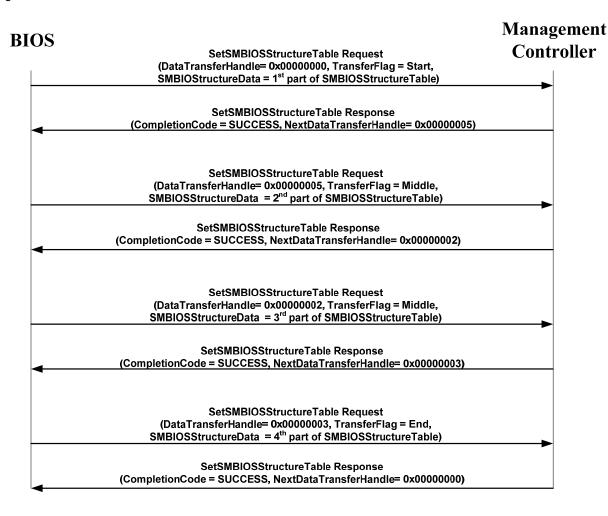
Figure 1 – Multipart SMBIOS Structure Table Transfer Using the SetSMBIOSStructureTable Command
