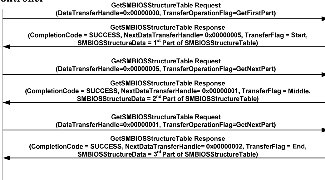
299 Figure 2 – Multipart SMBIOS Structure Table Transfer Using the GetSMBIOSStructureTable 300 Command
