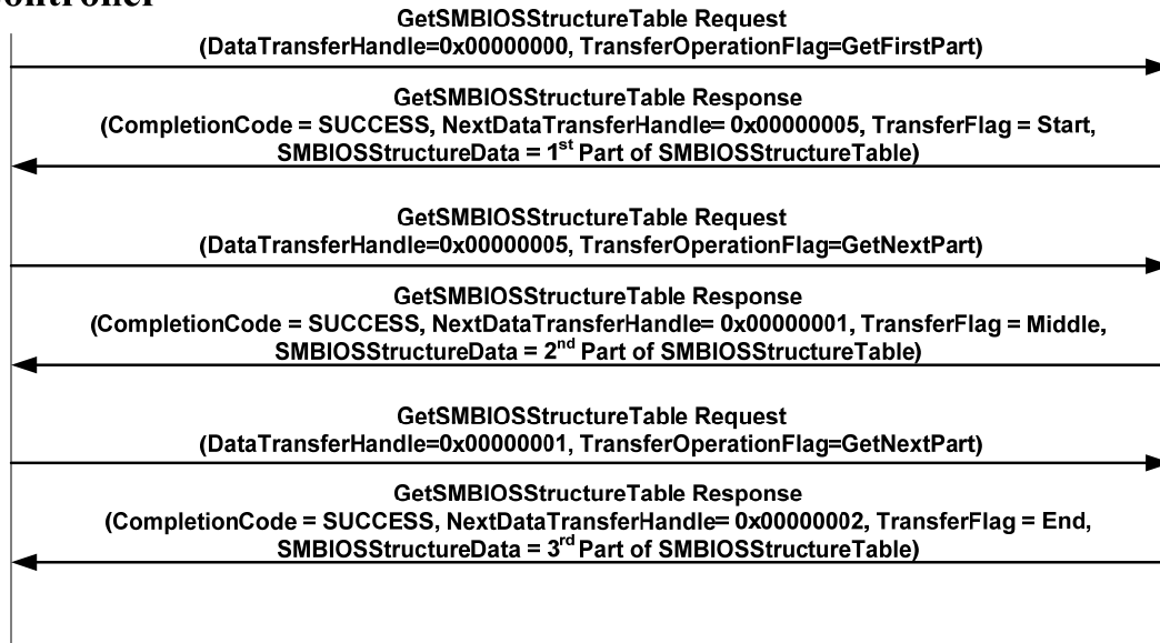
305 Figure 2 – Multipart SMBIOS Structure Table Transfer Using the GetSMBIOSStructureTable 306 Command
