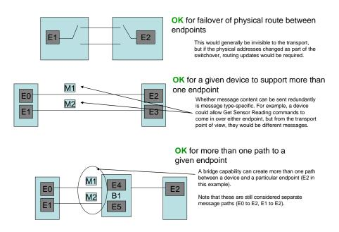
Figure 4 – Acceptable Failover/Redundant Communication Topologies
