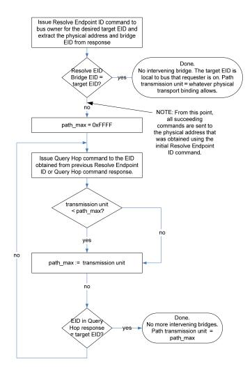
Figure 15 – Path Transmission Unit Discovery Flowchart
